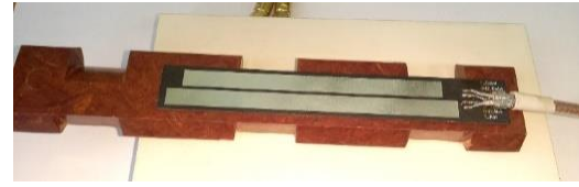
Fig.4 Example of electrocapacitive sensor for measuring stator bar vibrations
