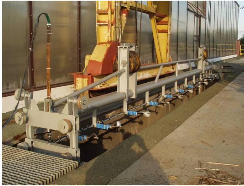
Fig. 8 Frames with fixed the current meters for traversing the hydrometric section.
